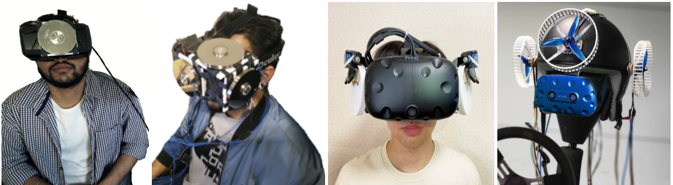
Fig. 4. Recent head-mounted disc-based gyroscopic haptic devices. Left to Right: GyroVR single axis, GyroVR triple axis from Gugenheimer et al. 2016, Kabuto from Tanichi et al. 2020 and Odin's Helmet from Hoppe et al. 2021.
