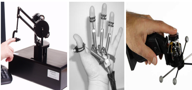
Fig. 2. The evolution of early handheld haptic devices that render resistances. Left to Right: PHANTOM (Massie, Salisbury, et al. 1994), Rutgers Master II (Bouzit et al. 2002), NormalTouch (Benko et al. 2016)
